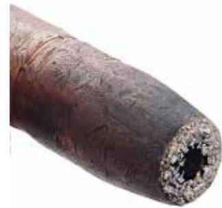
Nozzle fully clogged (not using E-WELD Nozzle)
